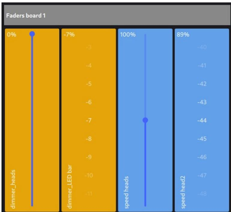
This board contains sliders and tumblers for dimmer control over channels, or speed control over scene buttons.
