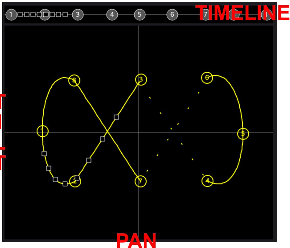
This curve is an example of curve for a pan/tilt movement.
