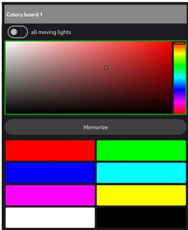
This board contains a color wheel with color memories to control the color of a group of fixtures.
