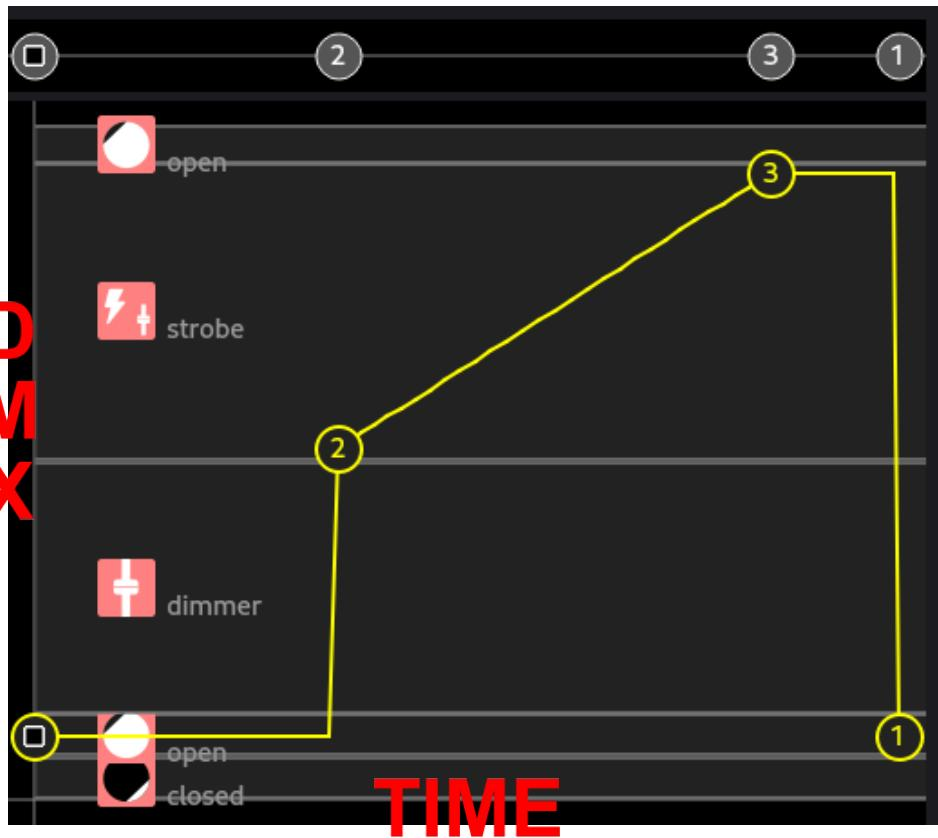
This curve is an example of curve for the channel « shutter ».
