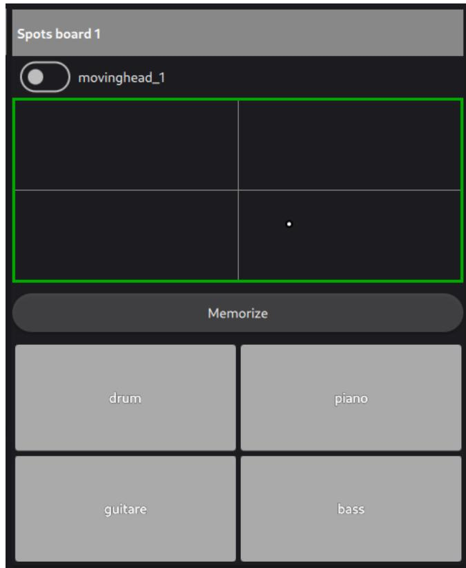
This board contains a pan / tilt section with positions memories to control the movement of a fixture.
